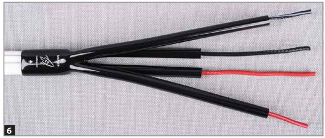
6. Push the pants on until they stop. The leads should be coming out of the ends of the legs.
